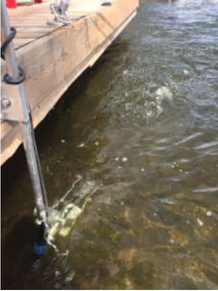
Pump shown in 45 degree position with water flow along dock edge.
